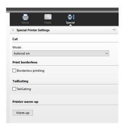
Tailgating is a feature which enables the HP Latex printers to print continuously from one job to the next.
